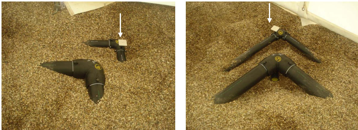
Figure 6. Electro-fusion couplers partly buried and exposed. A small metal electrode (arrowed) is attached to the metal coil within the coupler to enable the electrostatic potential to be easily measured.
